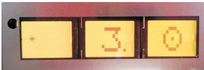
Figure 6. AK30/MK30 display with big numbers in yellowish colour in TABLES mode
