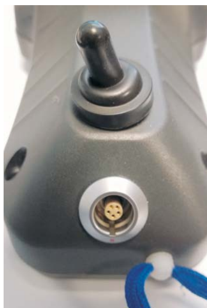
Figure 1. Power switch and charger connector for AK30, a LEMO OK connector
