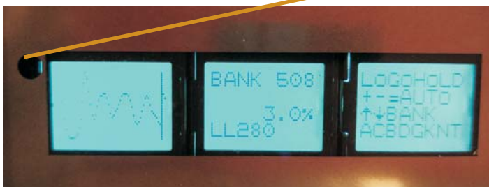
Figure 7. AK30/MK30 display with the trend curve and detailed information, in blueish colour in BANKS mode. The menu system is available at the same time.
