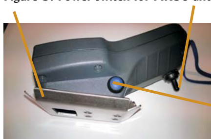
Figure 3. Power switch for AK30 and the PUS
