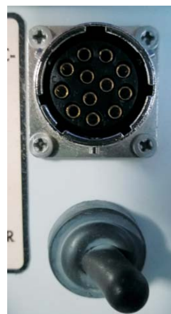
Figure 2. Power switch and power supply connector for AK40, a 12-pin ITT Cannon
