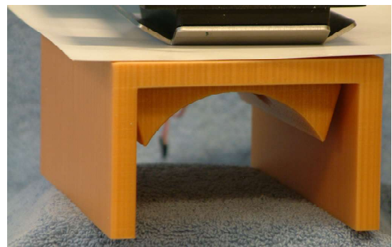
MK30R placed on the Sheet Calibrator back side and a sheet. Align the hole and the front panel asterisk
