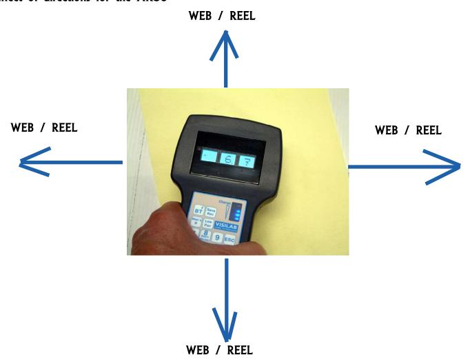
AK30 measurement can be done in any direction referring to the running web or reel.
