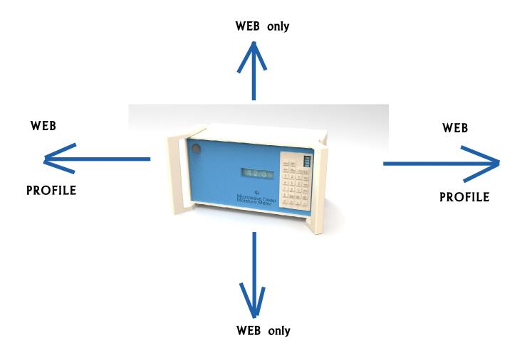
MK30R WEB measurement can be done in any direction referring to the running web or reel. It is insensitive to fiber orientation and web direction. Make sure the travel sensor is in its stall and not touching the paper surface. MK30R can be used for profile measurements in WEB setting by using the time base, usually 0.2 sec intervals.
